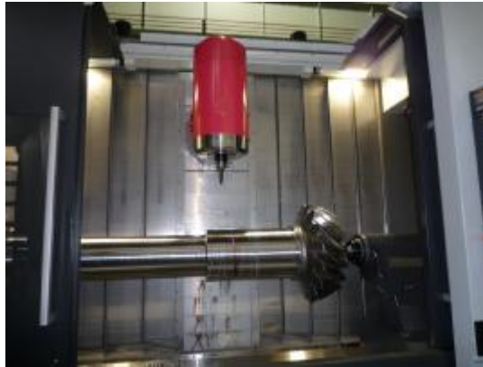
Fig. 8: Pinion-work on multi-tasking machine
