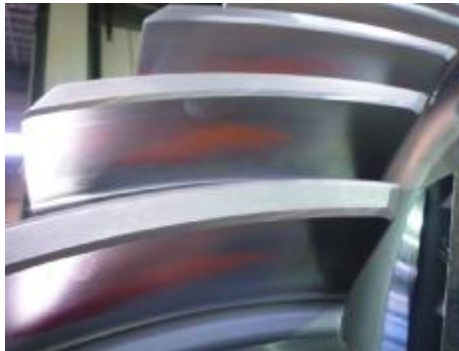
Fig. 12: Tooth contact pattern of coast side
