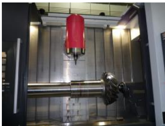
Fig. 8: Pinion-work on multi-tasking machine
