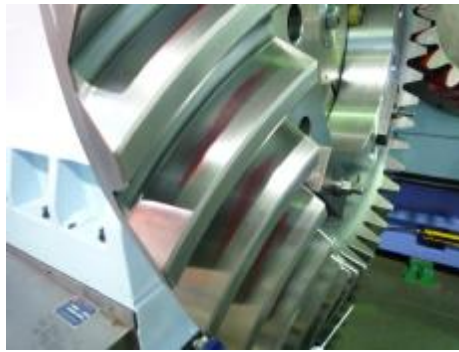
Fig. 11: Tooth contact pattern of drive side
