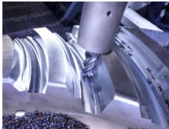
Fig. 7: Swarf cutting of gear
