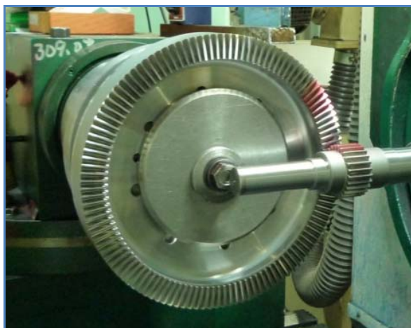
Figure 13. Face gear set on meshing tester
