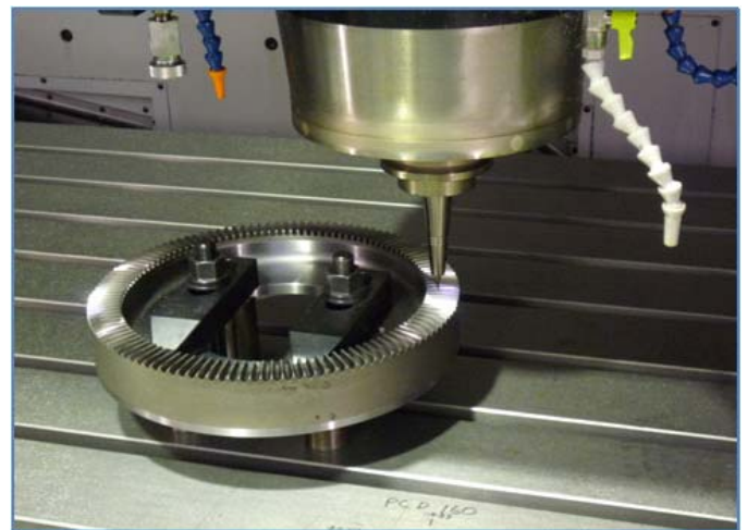
Figure 11. Machining of face gear
