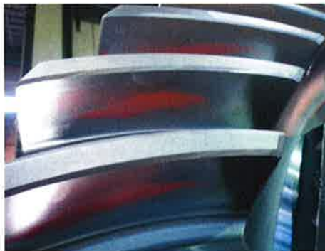
Fig. 12: Tooth contact pattern of coast side
