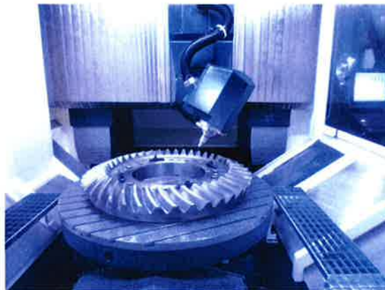
Fig. 6: Gear-work on multi-tasking machine
