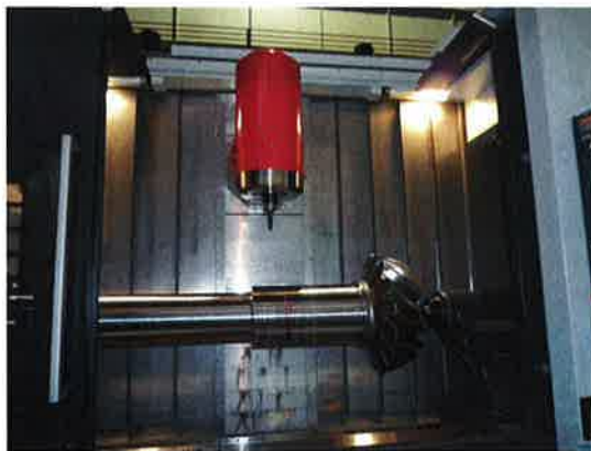
Fig. 8: Pinion-work on multi-tasking machine
