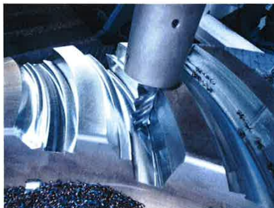
Fig. 7: Swarf cutting of gear
