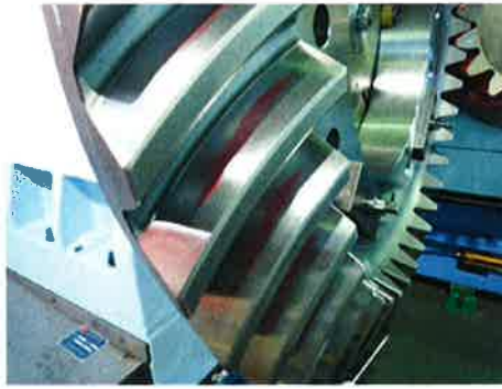
Fig. 11: Tooth contact pattern of drive side
